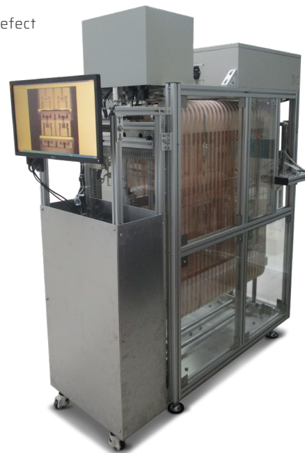
3D Post-Wirebond Reel-to-Reel Inspection
