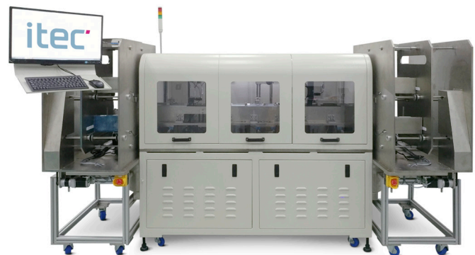
Strip-to-Strip Inspection after Plating
